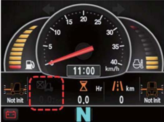
2) Vehicle that has applied the weight sensor (not set)
